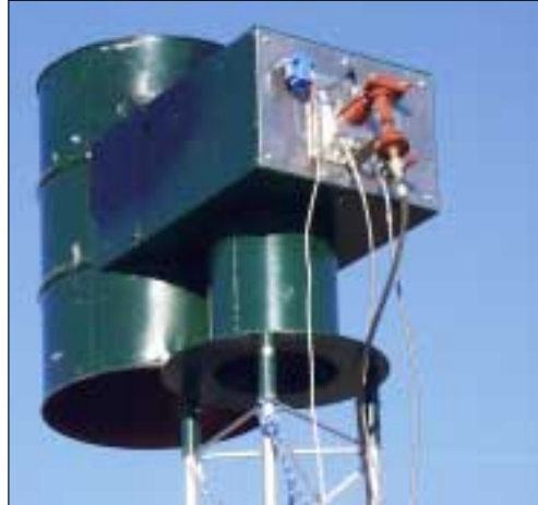
Silver iodide generators placed on mountaintops release condensation nuclei into passing clouds
